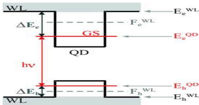
Figure 1: Energy diagram of the QD and WL system [23].
