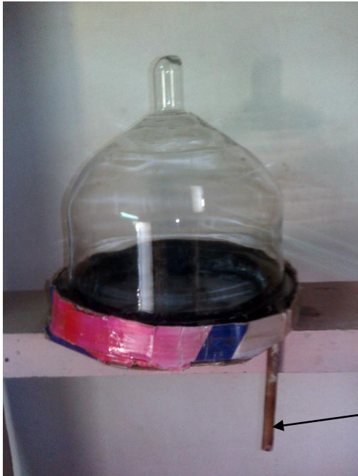
Figure 1: A photographic picture of the Hemispherical Solar Still (HSS)
